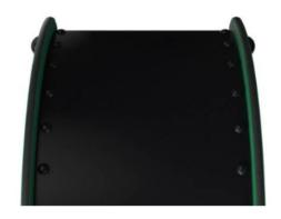
Membranes consist of friction-proof rubberized material of conveyor belt quality with excellent UV resistance. Embedded is a four-layered armouring made of woven polyester. The armouring and the two surface layers result in a total thickness of 9 mm.
