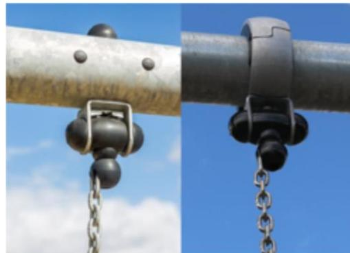
The swing hangers are made of high quality UV-stabilised nylon (PA6) housing with integrated lifetime sealed ball bearings. The height adjustable chains are fixed by a stainless steel hook with theft proof snake-eye bolt in a turn able anti twist housing. All seats with two chain fixation are available with either standard or anti-wrap suspension.
