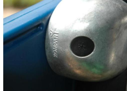
Panels and play activities are attached to the posts by pressure moulded lead free aluminium connectors with sealed bolt heads. The connectors are fastened to the post by a stainless steel strap and tightened by Loctite secured steel bolts.
