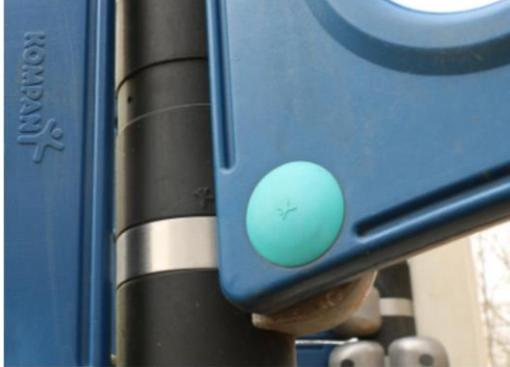
Main posts of 4" pre-galvanised inside and outside steel pipe with outer layer of 3mm thick PUR rubber. The PUR rubber is moulded directly on to the steel pipe to secure perfect adhesion for long lasting durability in all climates.
